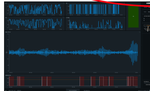
Rerun with measured motion data from vessels with parametric roll
