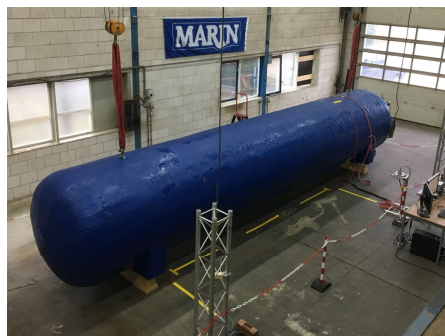
LNG-PITCH4 tests: instrumented prototype tank outside (1) and inside (2) the autoclave
