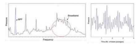
'ringing' effect, superimposed on the tonal components at blade passage frequency. Such a phenomenon has been observed in time traces of pressure signals measured with flush mounted pressure transducers on board passenger vessels.
