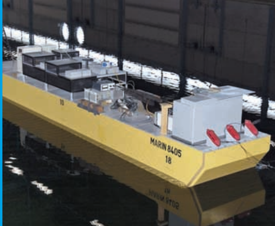
The Agbami FPSO (Chevron, Daewoo and SBM) during the towing (course stability and survival) tests in the Seakeeping and Manoeuvring Basin.
