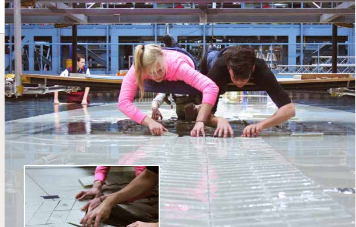
The artificial ice particles were placed in the channel by hand
