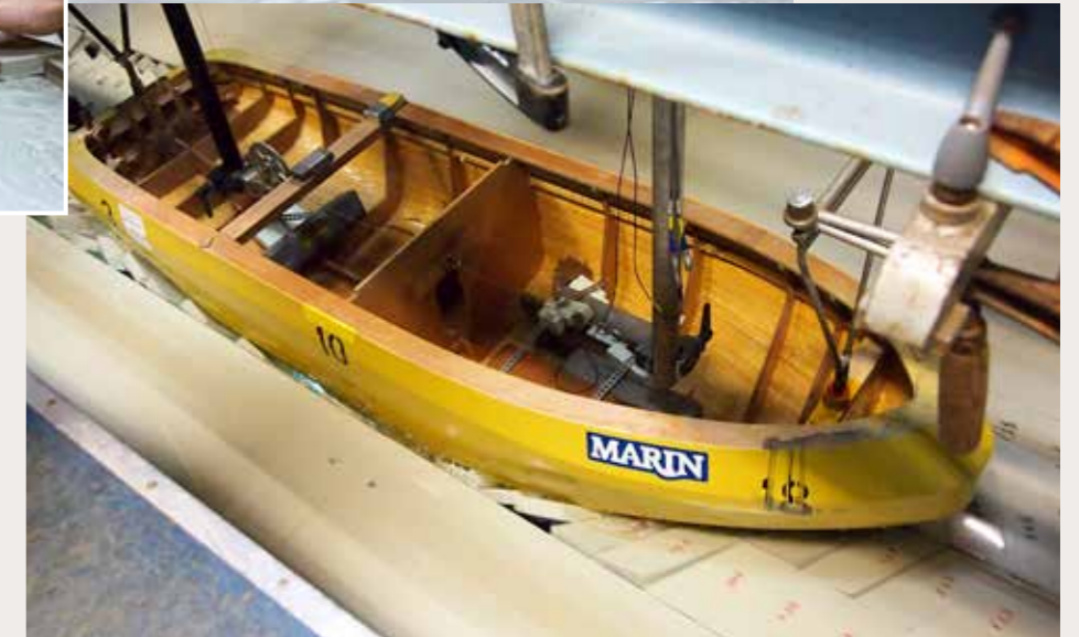
Model towed through the channel of artificial ice particles.
