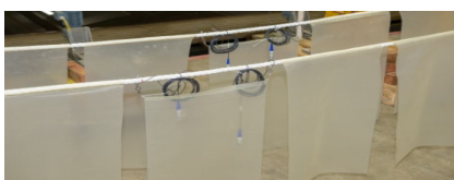
Seaweed modelled by using surrogate material. Top figure: fully moored multi long line model (scale 1:25). Bottom figure: Laminaria digitata surrogate (1:1)
